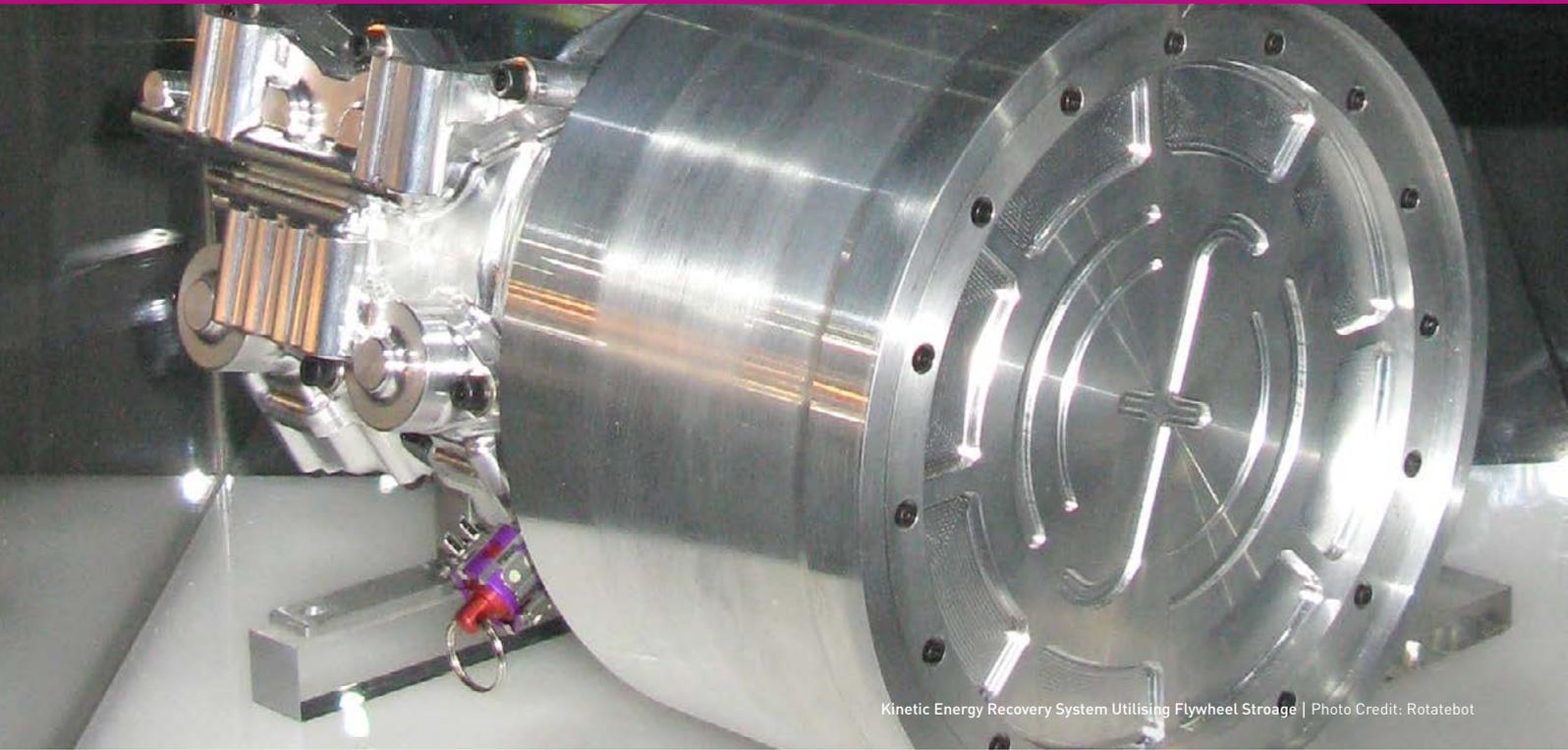
Kinetic Energy Recovery System Utilising Flywheel Storage | Photo Credit: Rotabot
